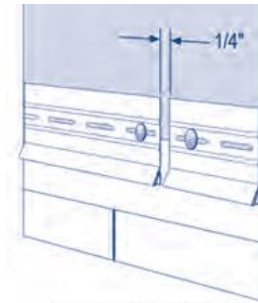
Starter trim installation
