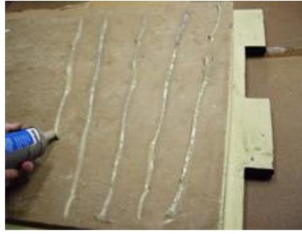
5.) Apply a bead of glue/adhesive to the perimeter of the back of the faux wood panel, roughly an inch from the edge.
