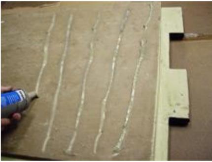
4.) Apply a bead of adhesive/glue to the perimeter of the back of the faux wood face, roughly an inch from the edge.
